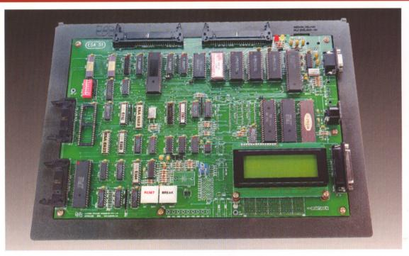
8051 family of microcontrollers and its derivatives are increasingly becoming popular for instrumentation and control applications due to its speed and powerful instruction set which are essential for real-time applications. This has created the need for a good trainer and development tools. ESA 51 (an advanced version of ESA 31) provides complete solution for this requirement. It can be used as a flexible instructional aid in academic institutions and a powerful development board in R&D Labs.
