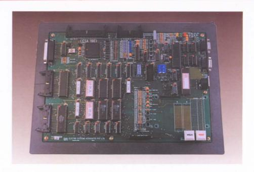
ESA 196 trainer is based on 80C 196 KB/KC microcontroller. ESA 196 trainer can be used as a flexible instructional aid in academic institutions and as a powerful development kit in R & D labs. ESA 196 can be used in realtime event control, motor control, high speed input / output operations and also in instrumentation.
