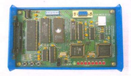
ESA MCB 51-2 Evaluation Board, a *special edition* of the successful ESA KEIL MCBx51 (now discontinued) with some advanced features, is meant for introducing the user to the 8051 family microcontrollers.
