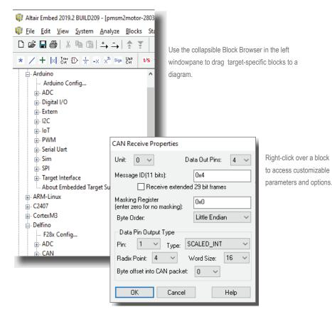
offer an extensive range of capabilities to support the development of systems with CAN communication.
