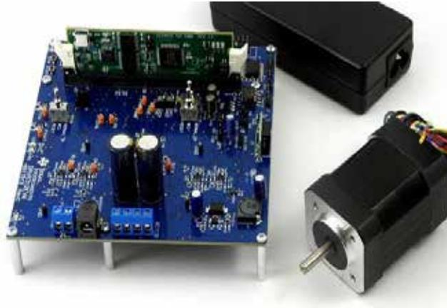
TI DRV8312EVM Sensorless Field-Oriented Control Motor Kit
